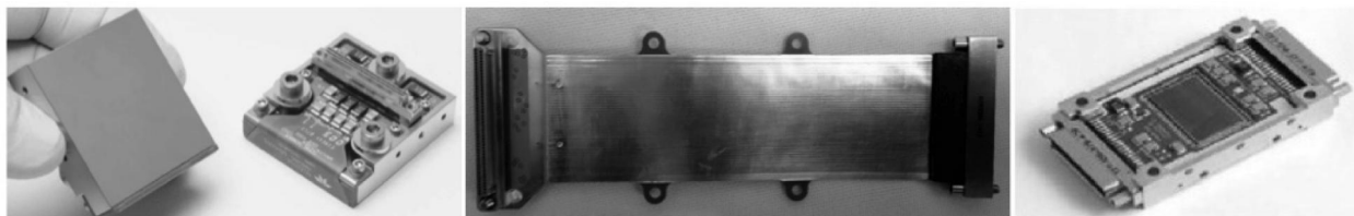
Figure 1. The SCA, CFC and SCE components comprising the SCS unit.
