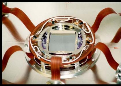
The Nov 2002 reduction in EPIC MOS (and RGS) operating T resulted in far fewer hot pixels, and decreased energy resolution degradation rates.
